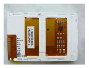
The display interface was measured using a HP (Agilent) 16-channel digital oscilloscope. (unfortunately a logic analyser was not available) The display commands and data are written in a 16-bit format like the example on the picture. A data bit is latched with the rising edge of the clock signal by the display controller.
